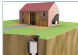
Bore hole collector
